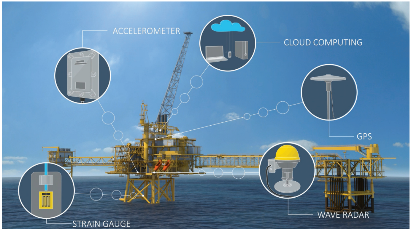
FIGURE 1. Exemplification of measurement equipment in a structural health monitoring system.
