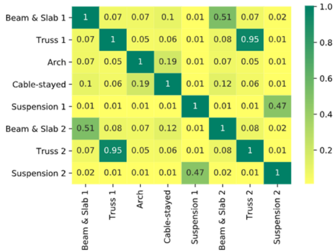
FIGURE 15. Illustration of how the PBSHM metric has allowed similarity measures between real bridge structures. The matrix shows the similarity scores between IE/AG models of a set of eight bridges. The score is normalised to unity for a perfect match (the diagonal); note the high scores for the pairs of beam and slab bridges, suspension bridges and truss bridges.
